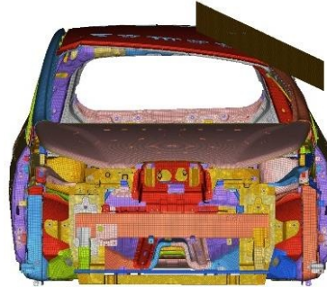
Fig.4 Analysis of roof crush resistance with CFRP side Beam
